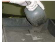
Cover "green" part and bronze infiltrant with alumina powder
